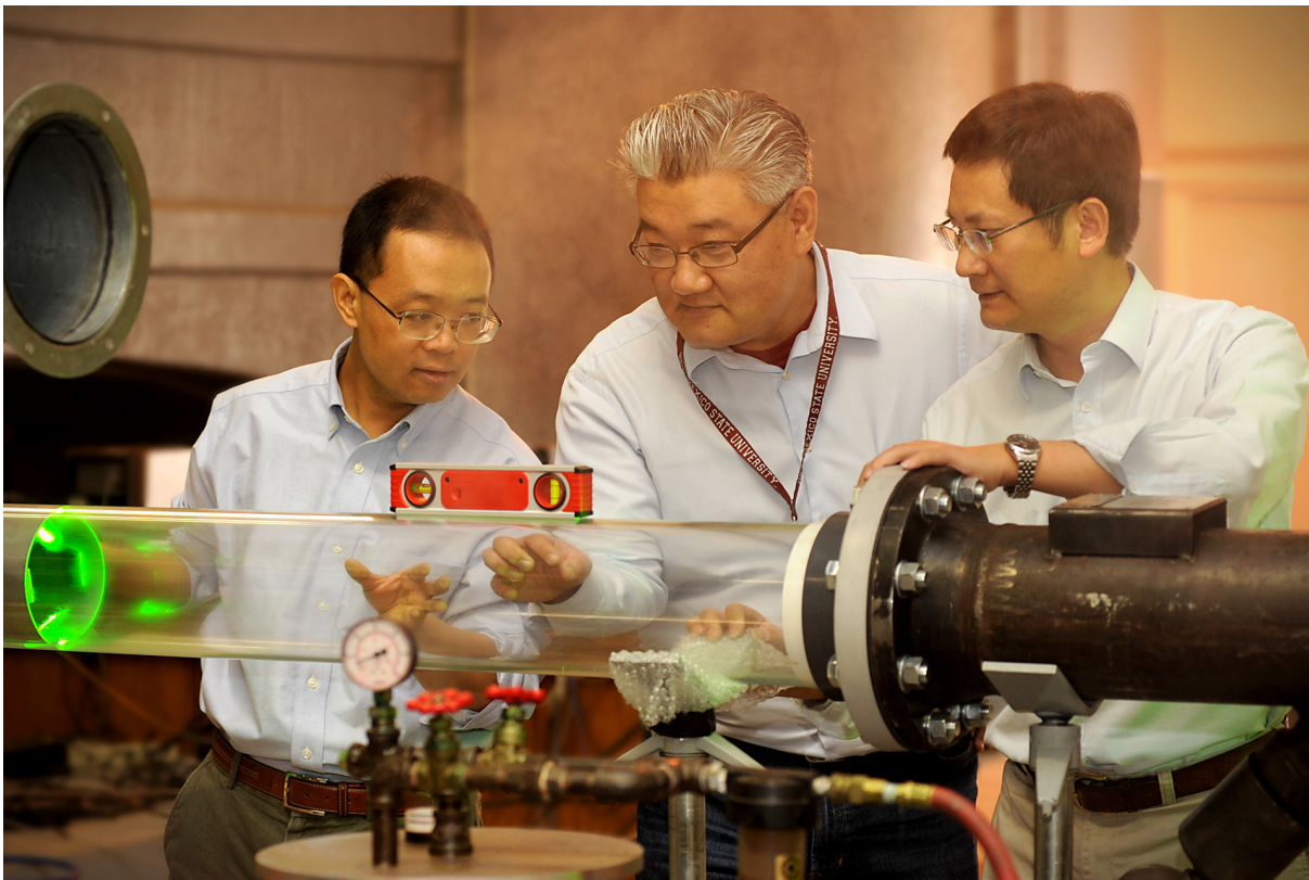
NMSU Mechanical and Aerospace Engineering Professors Mingjun Wei (left), Young Lee, and Fangjun Shu measure flow downstream turbulence generated in a diesel engine intake using particle image velocimetry system (Photo by Darren Phillips).
